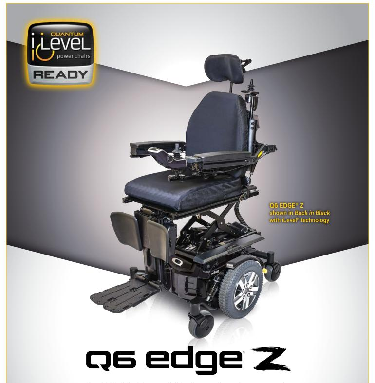
The Q6 Edge® Z utilizes powerful 4-pole motors for maximum torque and Mid-Wheel 6® design for aggressive outdoor performance and precision indoor maneuverability. The Q6 Edge® Z accepts a broad range of exclusive seating and electronics options for unmatched adaptability and rehab capability, and is available with our iLevel® technology.
