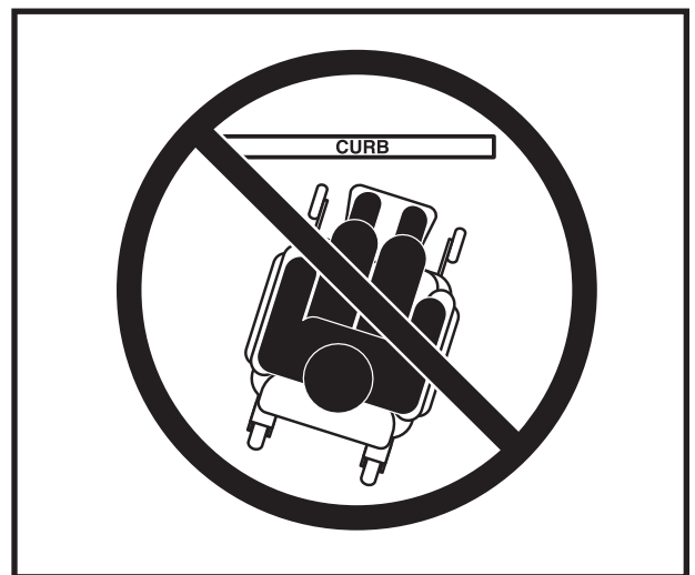
Figure 5. Incorrect Curb Approach
